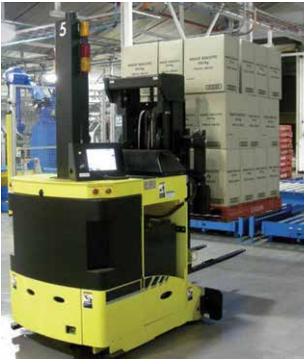
Figure 4: Automated Guided Vehicle. Source: IndiaMart
